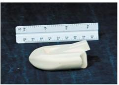
Syntactic foams are a unique combination of hollow spheres, a resin matrix, and other additives. When combined and processed properly, the constituents form a lightweight homogeneous material having high compressive and hydrostatic strengths. This yields a product able to withstand the extreme hydrostatic pressures experienced by today's manned and unmanned subsea vehicles.
