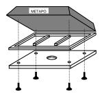
Distance holder or distribution channels on base plate
